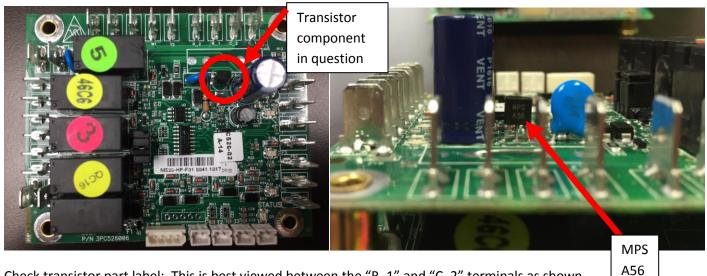
Check transistor part label: This is best viewed between the "R\_1" and "C\_2" terminals as shown
